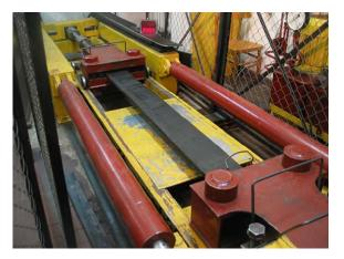
Fig. 2. Tensile testing machine ZP-40 for belt joints
